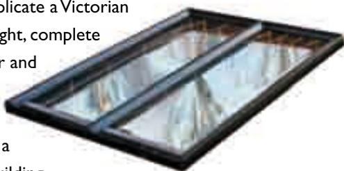
This makes it a very unobtrusive termination for the SunPipe system. The rooflight incorporates a sealed double glazed unit with an outer layer of 4mm toughened glass, a 12mm air gap and a 4mm K toughened inner panel
