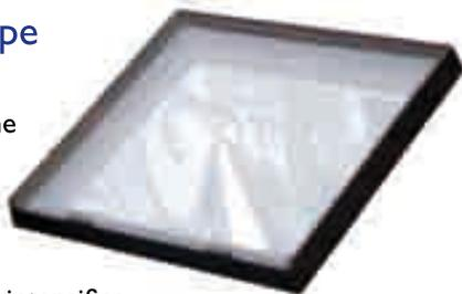
The Square SunPipe rooflight frame measures 610 x 610mm with a glass area of 505 x 505mm. The mirror finish square adaptor inside reduces the size to 500 x 500mm and this is connected to the SunPipe tube. The system can fit 9" (230mm), 12" (300mm), 18" (450mm) and 21" (530mm) SunPipe tubes. The SunPipe adjustable elbows enable the system to fit any angle of roof.
