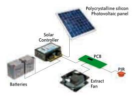
The ABS unit houses fully sealed solar batteries, which run at 12V. These batteries are designed to allow operation for up to 7 days without any charge from the solar panel.
